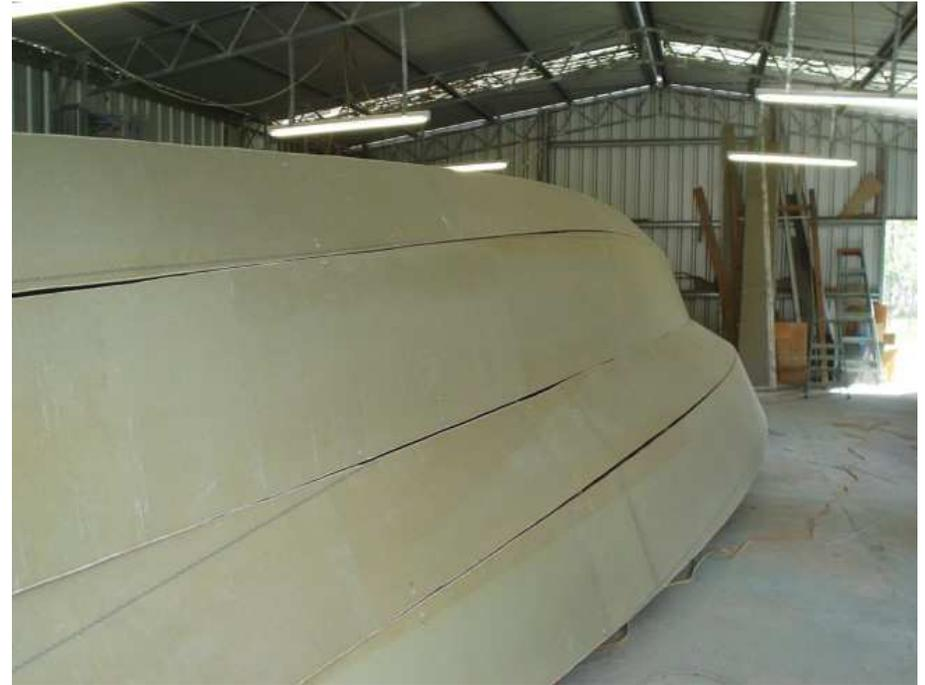
When all the panels are attached bog between the joints and sand. The joints can then be taped with glass tape (covered with peel ply. If the boat is plywood then the boat can be covered with glass and peel ply. The stem is clamped as the float and glued and taped.
