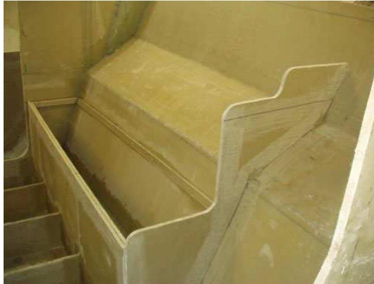
Horizontal shelves to the sides were added for a navigation station and a shelf for the portable fridge and platform for the porta-potti.
