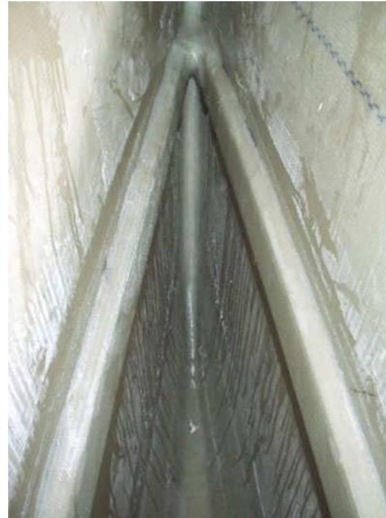
The bulkheads are temporarily held in place and taped. A couple of deck beams are added to support the deck.
