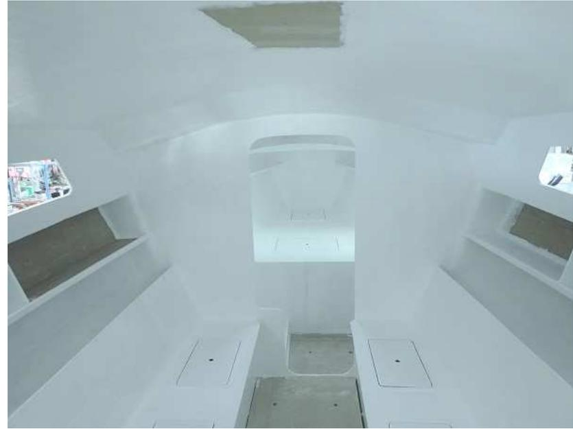
The cockpit was built with number 4 and number 6 bulkhead used as supports for the cockpit seats.
