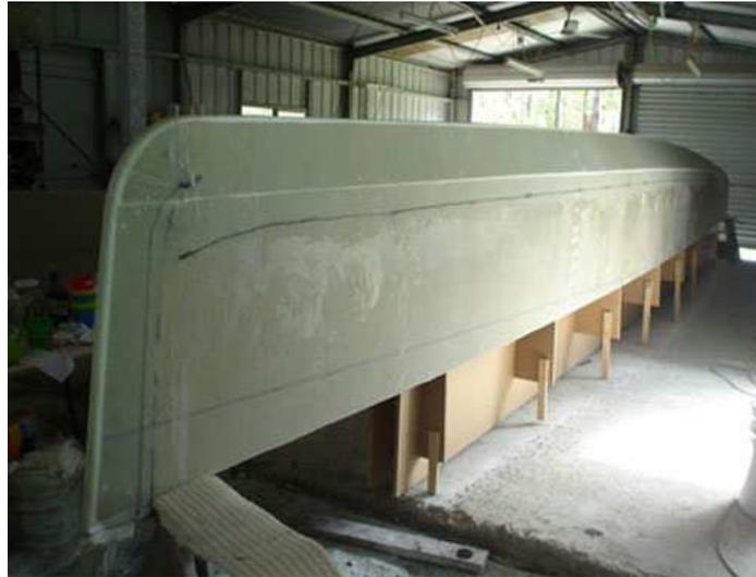
The float is turned and joints taped on the inside (pre-laminated panels) or glassed overall (plywood). It is easier to tape the inside joints using a wet fillet before taping.
