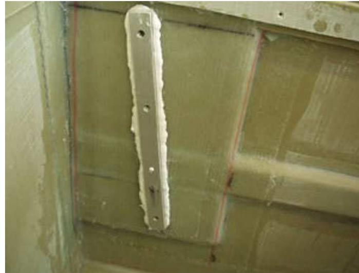
Glue was liberally spread on top of bulkheads, deck beams and in-wales. Deck was added using metal strapping to hold it in place.
