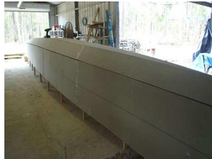
The stem of the float is clamped together and bog is applied to all joints.
