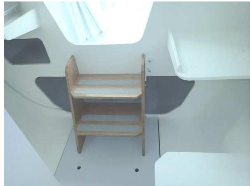
The inside has been polyester Flo-coated white, applied with a mohair roller. If any modifications need to be made or additions laminated on, the polyester flo-coat will be easier to prepare than grinding paint back to the fibreglass.
