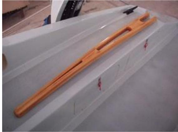
The tiller is made from laminated hoop pine and varnished.
