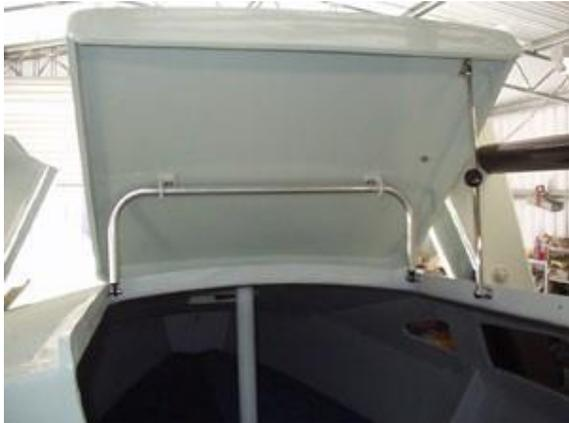
Forward hatch was attached with Sikaflex and stainless screws.
