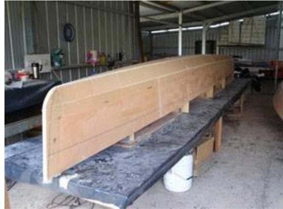
The floats are removed from the frame and taped inside. The floats were levelled and the bulkheads trimmed to fit. All the bulkheads are taped in the floats. A stringer was added in the centre to help the deck hold its shape
