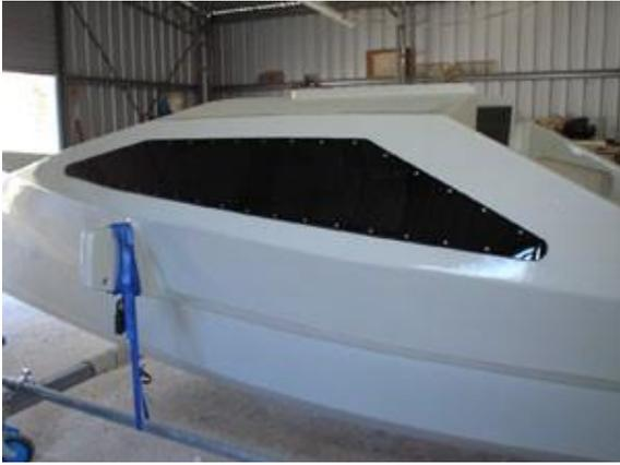
The locker covers are painted, trimmed and attached with hinges. Small pieces of stainless steel are bent and added as latches with some spectra rope added.
