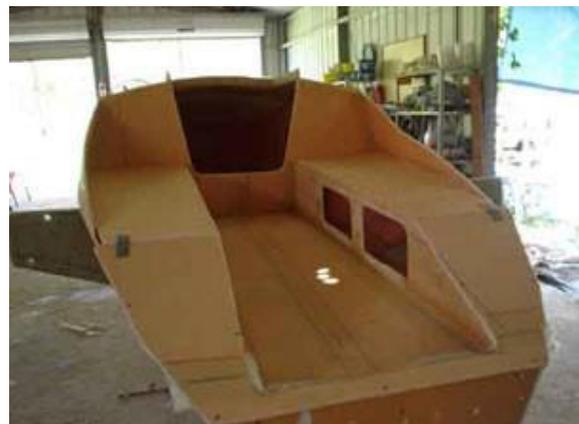
Cockpit is taped. Edges of the cockpit are rounded off using a long board and taped. Plywood inserts are added as stops for the locker doors.
