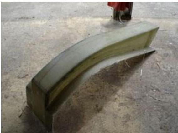
When the beam is removed from the mould it can be trimmed with a diamond disc in an angle grinder.
