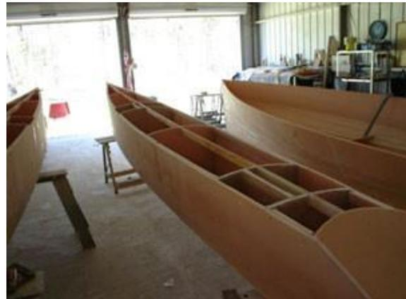
The laminated panels are too stiff to bend over the deck shape. We attached scraps of foam on the outside of the hull to temporarily hold the deck. The foam was joined to the right length and drywall screws were used to attach the deck foam to the hull. Care was taken to not screw into the hull itself. The deck was laminated with glass cloth and resin on the outside. When the glass hardens still attached to the scrap foam. The scraps were removed and the inside of the deck was laminated.
