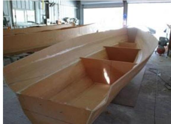
The main beams are taped in. A ring of glass is laminated around the main hull from side to side on the forward and aft beams.
