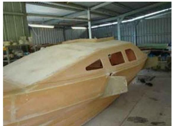
A plywood template for the window shape is temporarily attached and the shape drawn on the cabin sides. Holes for the windows are cut and the foam removed around the edges and filled.
