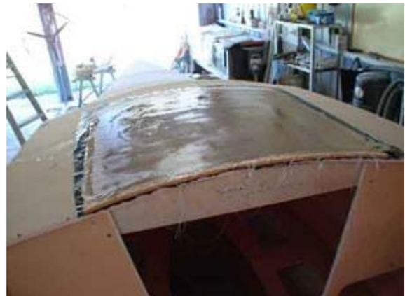
This is a good time to make a hatch top. Plastic is laid over the cabin roof and foam is temporarily screwed down and glassed on the top surface.
