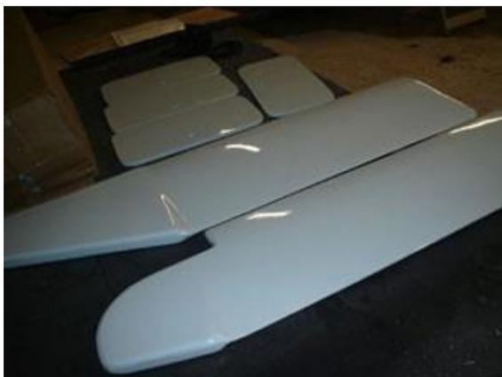
A rudder head is made using a form ply mould. The mould is waxed and layers of glass are wrapped around the mould. Peel ply was used on the outside to minimise the time spent finishing the head. After the mould was removed the rudder head is trimmed to shape and joined to the rudder blade with a stainless pivot pin. The pintles are screwed onto the blade to match the gudgeons on the stern
