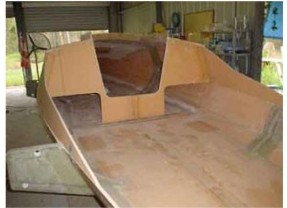
The hatch is finished off with scraps of laminated foam added around the edges and taped. The edges of the foam are removed and filled with filler.
