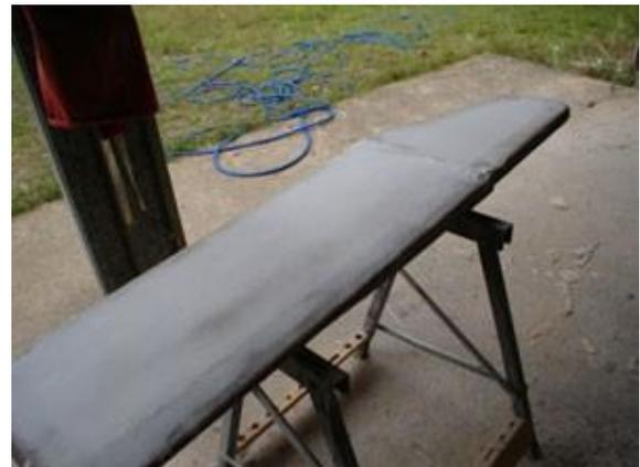
The centre board and the rudder are made using layers of plywood. Two pieces of 12mm plywood are laminated using a couple of layers of glass cloth and epoxy resin between. When the board is shaped the glass inside gives a sharp finish to the trailing edge directions in the plans.
