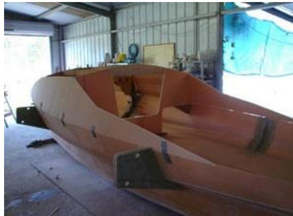
The cabin sides are attached to the frame and the other cabin panels with metal straps. Foam is bent over the frame and attached to temporary pieces of foam attached to the cabin sides. Glass cloth is laid over the foam and wetted out with resin. We use peel ply as well to cut down on finishing later. The edges of the cabin sides and roof are then taped.
